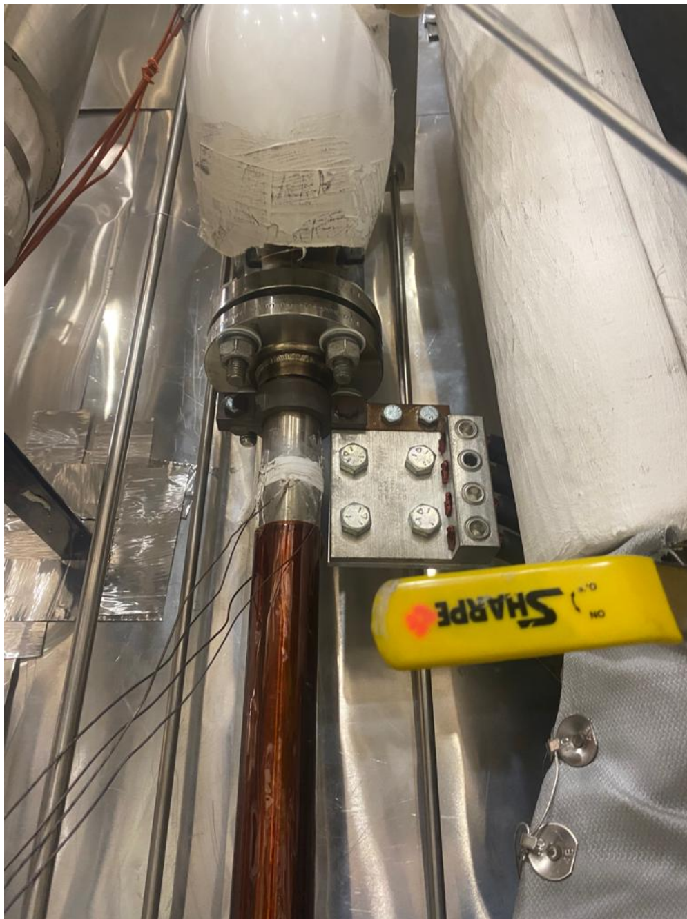
Figure 3.9: CIET's Heater with Emphasis on Top Head, brown material on heated section is Kapton tape to allow Infra Red Imaging
