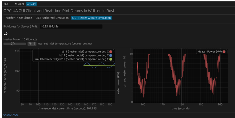
Figure 6.26: Oscillatory Behaviour Observed during Early Iterations of PID Control based SNF
