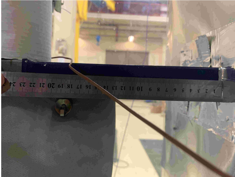
Figure 2.29: Photograph of showing Support Structure Length of about 23 cm in CIET near DHX Branch, Credit Omar Ashraf Alzaabi
