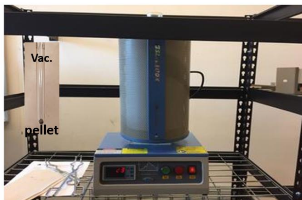
Figure 6. Vertical tube furnace used in this work – inset shows a sealed tube holding the pellet
