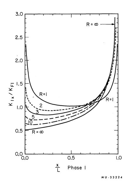
Fig. 3. Local mass transfer rates, Model 1.
