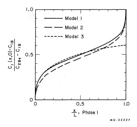
Fig. 6. Interfacial concentrations; comparison of models. R = 1.
