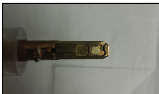
Figure 2.4: The graphene liquid cell is placed in the TEM holder in exactly the same way as a normal TEM grid.
