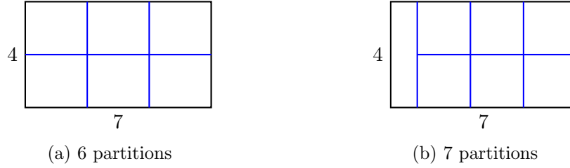
Figure 3.5: Examples of Partitioning a 2D block of size 7 \times 4 with IF. For 6 partitions, the factorization close to the length ratio 7 : 4 is 6 = 3 \times 2 . For 7 partitions, the leftmost sub-block is cut off to resolve the prime number. The remaining sub-block is factorized into 6 partitions based on the length ratio 6 : 4 .
