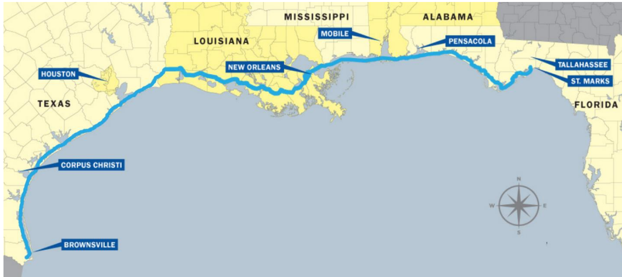
Figure 4.1. The Gulf Intracoastal Waterway is an inland, man-made waterway along the coast of the Gulf of Mexico that runs over 1,100 miles from the southern tip of Texas through the Florida panhandle. It is dredged on an ongoing basis to maintain sufficient depth for commercial and recreational marine transportation (image: Texas Department of Transportation, 2020). 35
