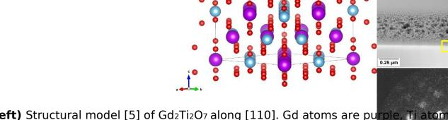
**Figure 1 (left)** Structural model [5] of Gd<sub>2</sub>Ti<sub>2</sub>O<sub>7</sub> along [110]. Gd atoms are purple, Ti a red. Note the different chemical compositions of alternating {22�2}-type planes.
