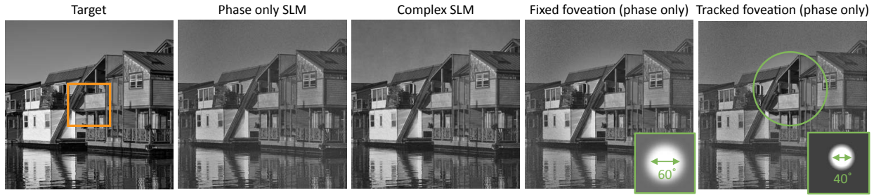
Figure 7.8: We propose three methods to further improve contrast for 16\times étendue enhancement beyond the performance of our baseline frequency constrained method (shown in second panel). First, with emerging complex-valued SLM technology, image contrast can be improved over the whole FoV. Second, since the eye tends to rotate only within a limited range before the head moves, in a 120^\circ display a large portion of the FoV is almost always in the periphery. Therefore, we can improve contrast in the center by applying our spatial constraints in a fixed foveation pattern that does not require eye tracking. Finally, if eye tracking is available, our spatial constraints can be used to improve quality in a dynamically changing subregion, highlighted by the green circle. The orange box indicates the native FoV, and the spatial maps used in the foveated simulations are shown in the insets. Floating houses source image by Madeleine Deaton (CC BY 2.0).
