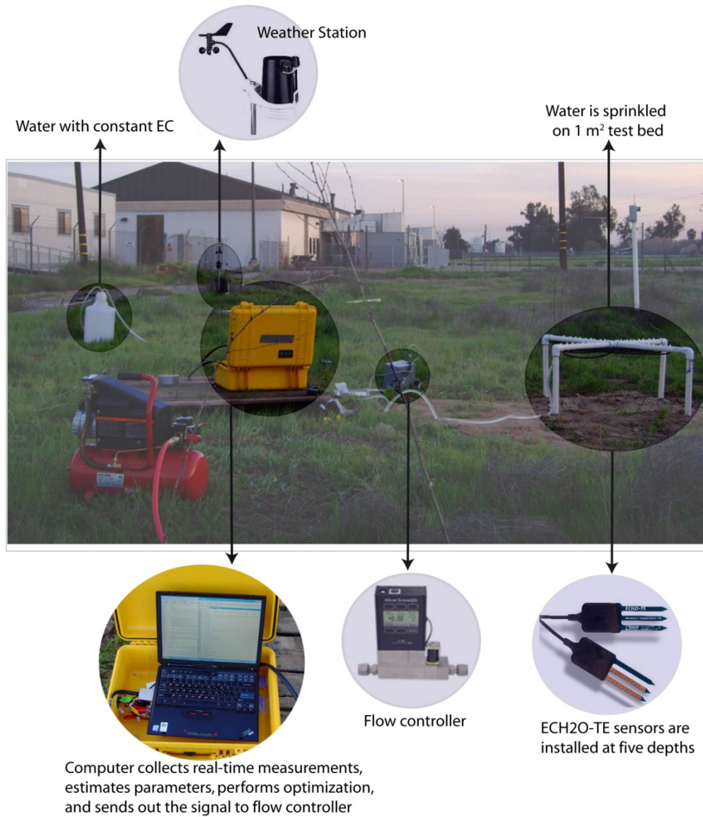
1 2 Figure 3. The pilot-scale closed-loop irrigation observation and management system constructed 3 for testing the RHC algorithm (see text for component details). 4
