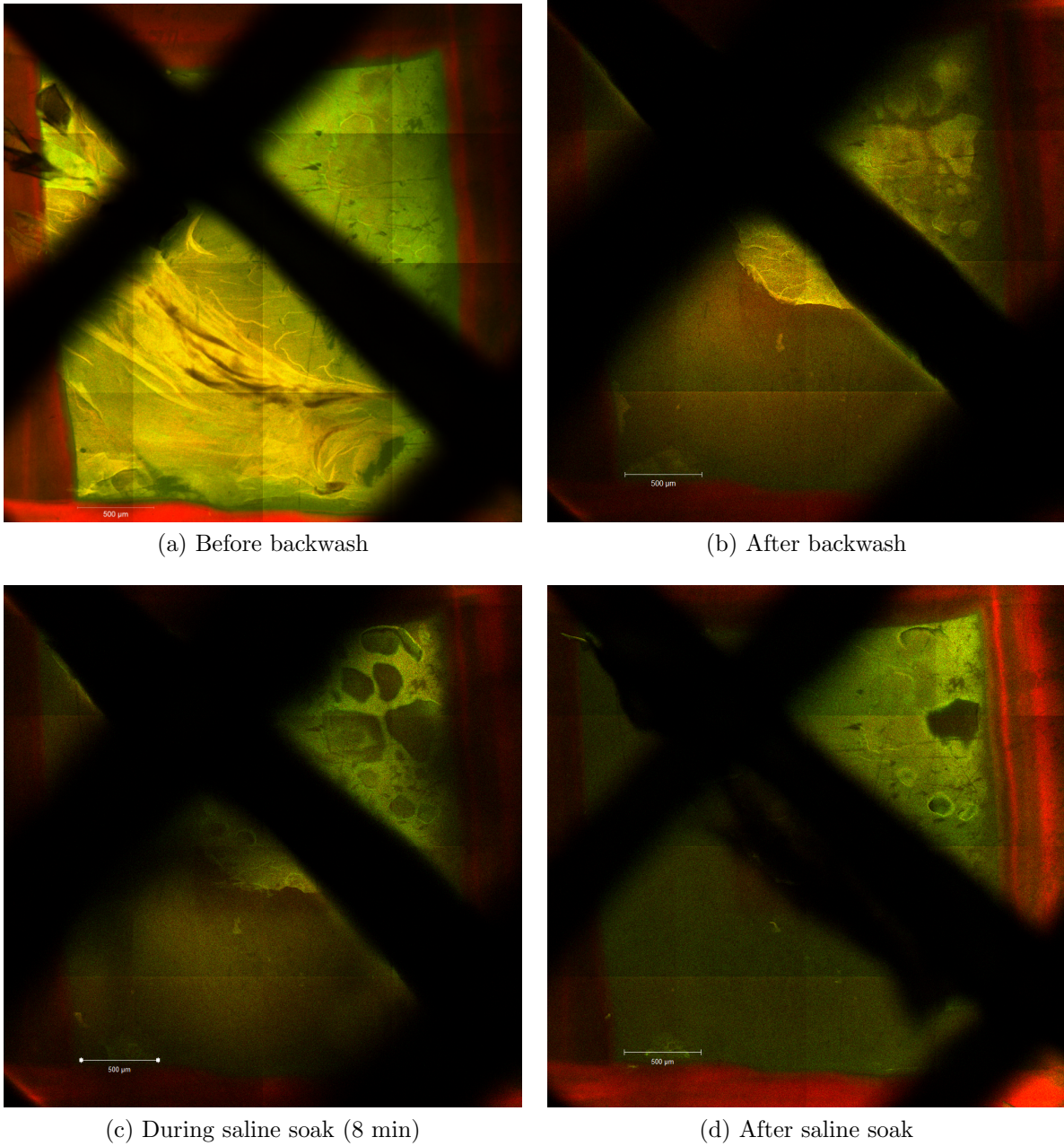
Figure B.23: Backwashing and a saline soak were performed sequentially on a UF membrane fouled for 2 d. (a) and (b) show the effect of a backwash, while (c) and (d) show the effect of a saline soak.
