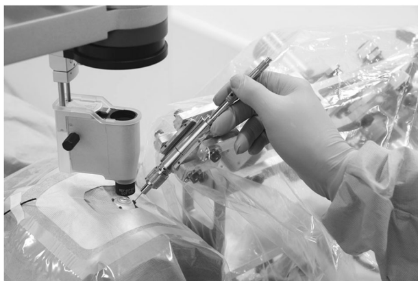
Fig. 5 Co-manipulator Robot. The intraocular robotic system of the Catholic University of Leuven, Belgium [17].
