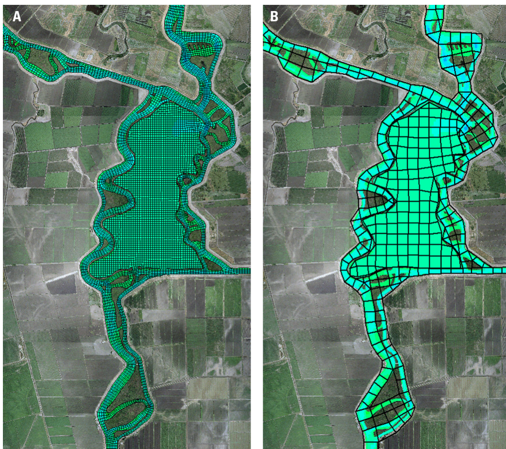
Figure 2 Comparison of model grids in the region of Mildred Island from (A) the high-resolution UnTRIM Bay–Delta model grid; (B) the coarse-resolution UnTRIM Bay–Delta model grid
