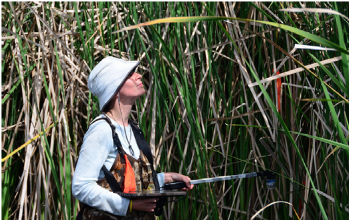
Iryna prepares to take hemispherical fish-eye images with a CI-110 Plant Canopy Imager in a tall reed canopy. Courtesy photo
