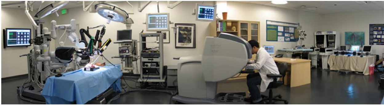
Figure 9-4: Center for Advanced Surgical and Interventional Technology dry lab at UCLA. Collaborative efforts between clinicians and engineers have led development of an integrated surgical suite with robotic surgical simulators, intraoperative ultrasonic imaging, and diagnostic MRI-ultrasound fusion devices.
