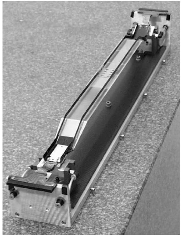
Fig. 19. Photograph of an SVT arch module in an assembly jig.
