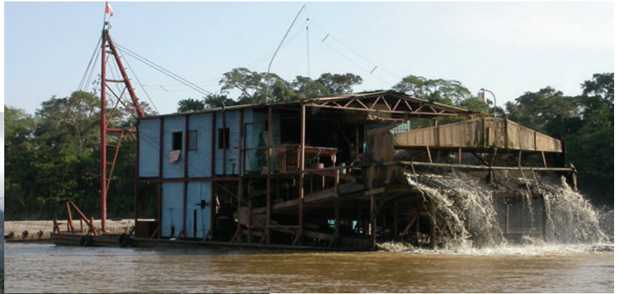
Figure 3 (right): A dredging operation in the MDD. The boat collects and rinses rock in search of gold, then dumps it back into the river. Photo courtesy of Dr. Donald C. Taphorn.
