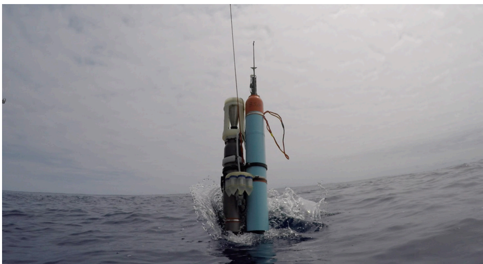
Figure 2: A CFE robot breaks the surface of the ocean as it is launched. It is ready to monitor how much carbon the Pump is sending downwards.
