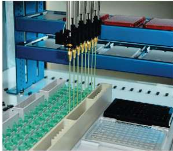
Figure 1.1 An example a high-throughput assay. Pipetting robots are used to reproducibly mix reagents in well plates.
