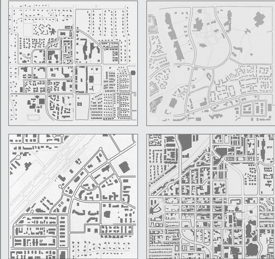
This study compared mile-square sections of four mixed-use districts in Scottsdale, Arizona. Clockwise from top left: an older neighborhood commercial district, a newer district with power retail and offices, downtown and a light-industrial/corporate district. Illustrated here are pedestrian networks; the study also documented block patterns, property lines, building figures, surface parking and clusters of similar building types. The project replicated methods done by
