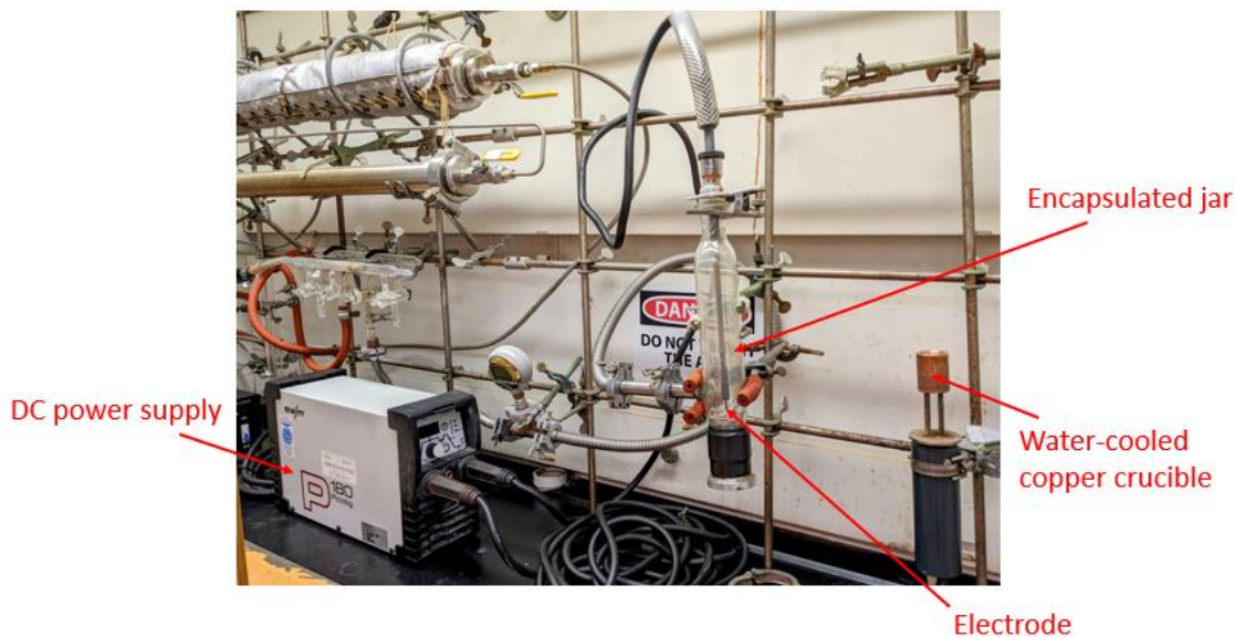
Figure 2.2: Arc melting furnace used for experiments.
