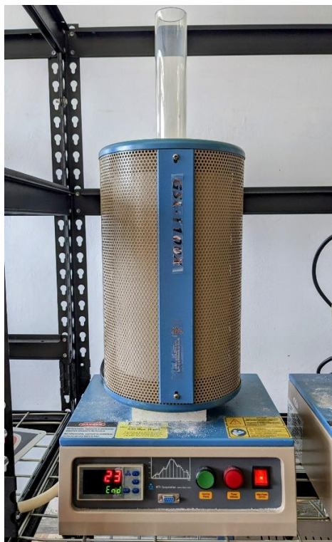
Figure 2.3: Vertical tube furnace used for experiments.
